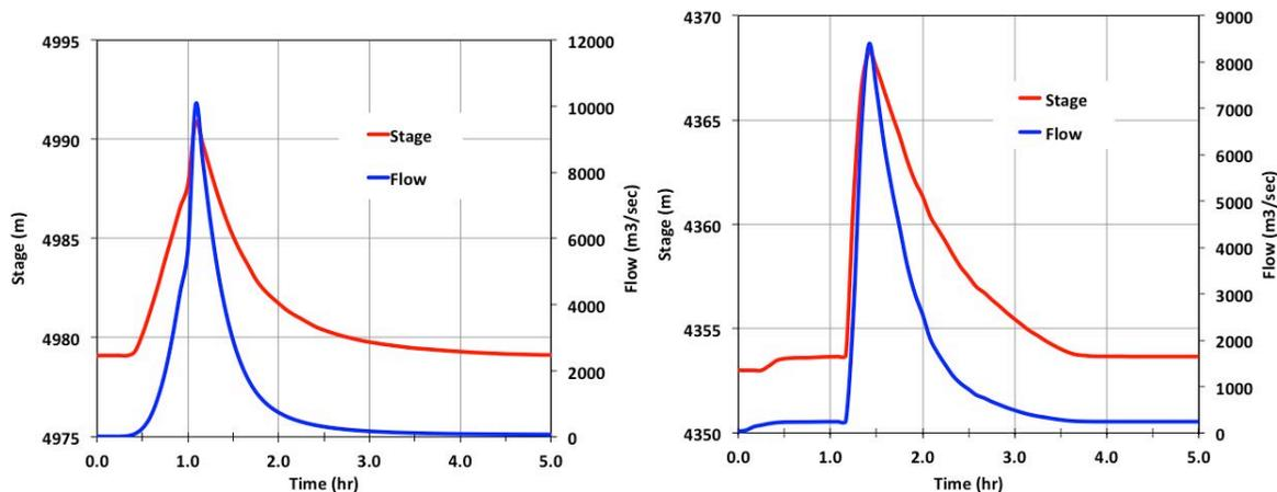
Figure 4. Left: Hydrograph at Imja Lake. Right: Hydrograph at Dingboche, 8.4 km downstream of Imja Lake outlet.
